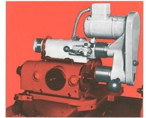
Face grinding device to square a face to a ground bore.
